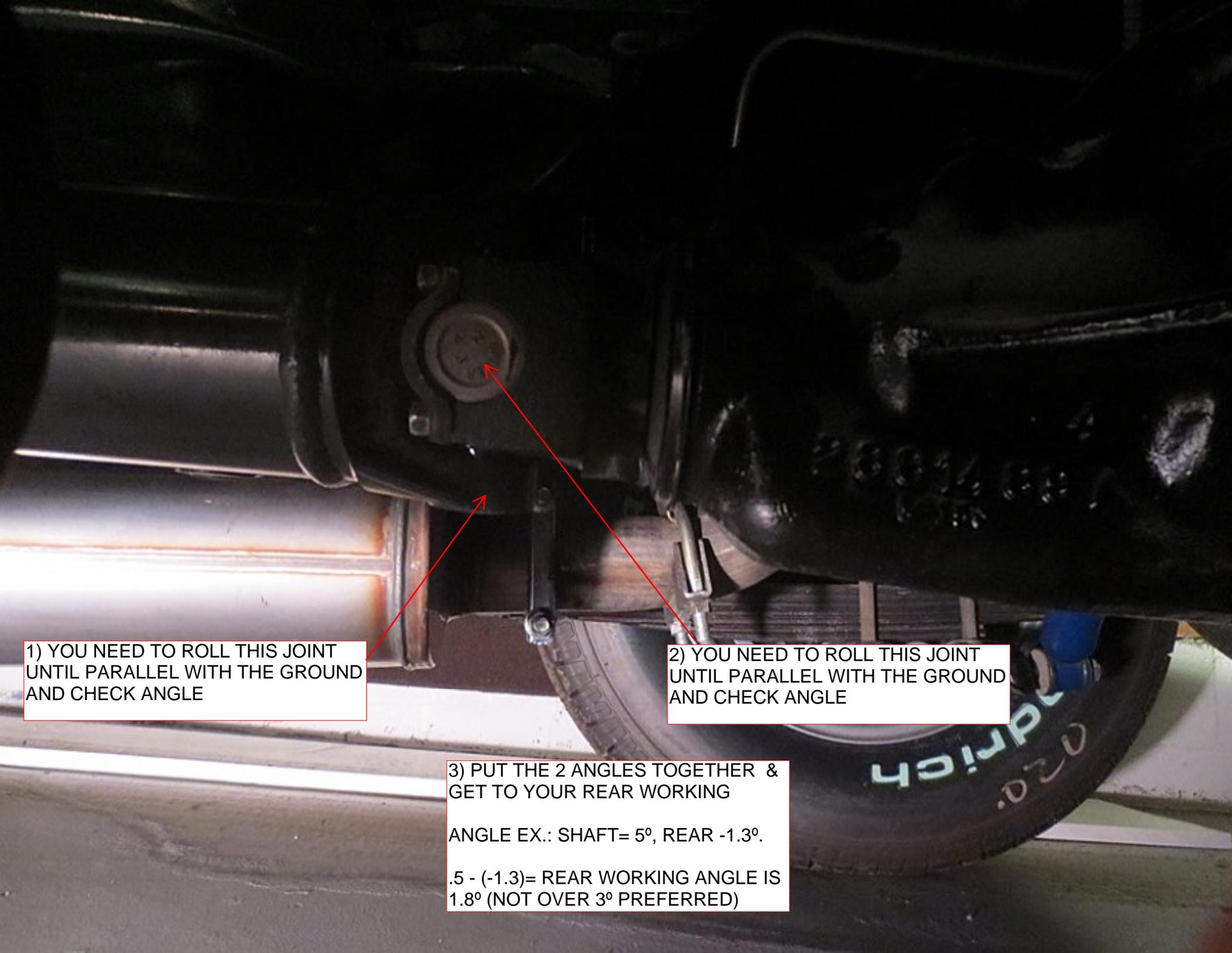
1) YOU NEED TO ROLL THIS JOINT UNTIL PARALLEL WITH THE GROUND AND CHECK ANGLE
