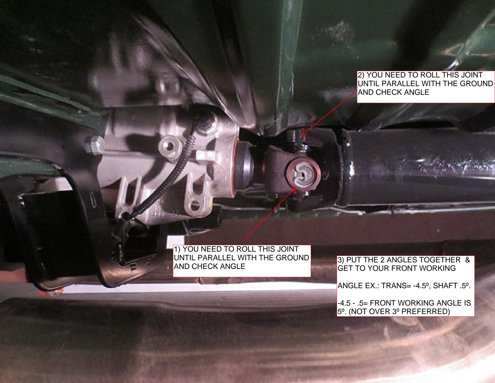
2) YOU NEED TO ROLL THIS JOINT UNTIL PARALLEL WITH THE GROUND AND CHECK ANGLE
